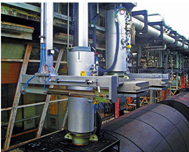
↑ On-spot rail car loading
