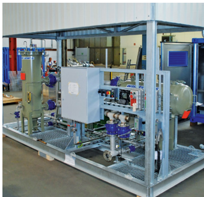
↑ Refueller loading skid
